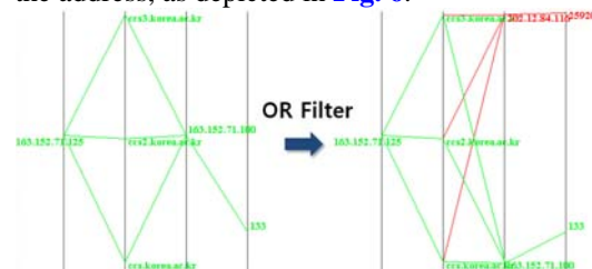
Fig. 6. Filtration effect on a DNS cache poisoning
